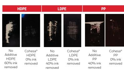
Tested by ASTM D3359: Standard Test Methods for Rating Adhesion by Tape Test
