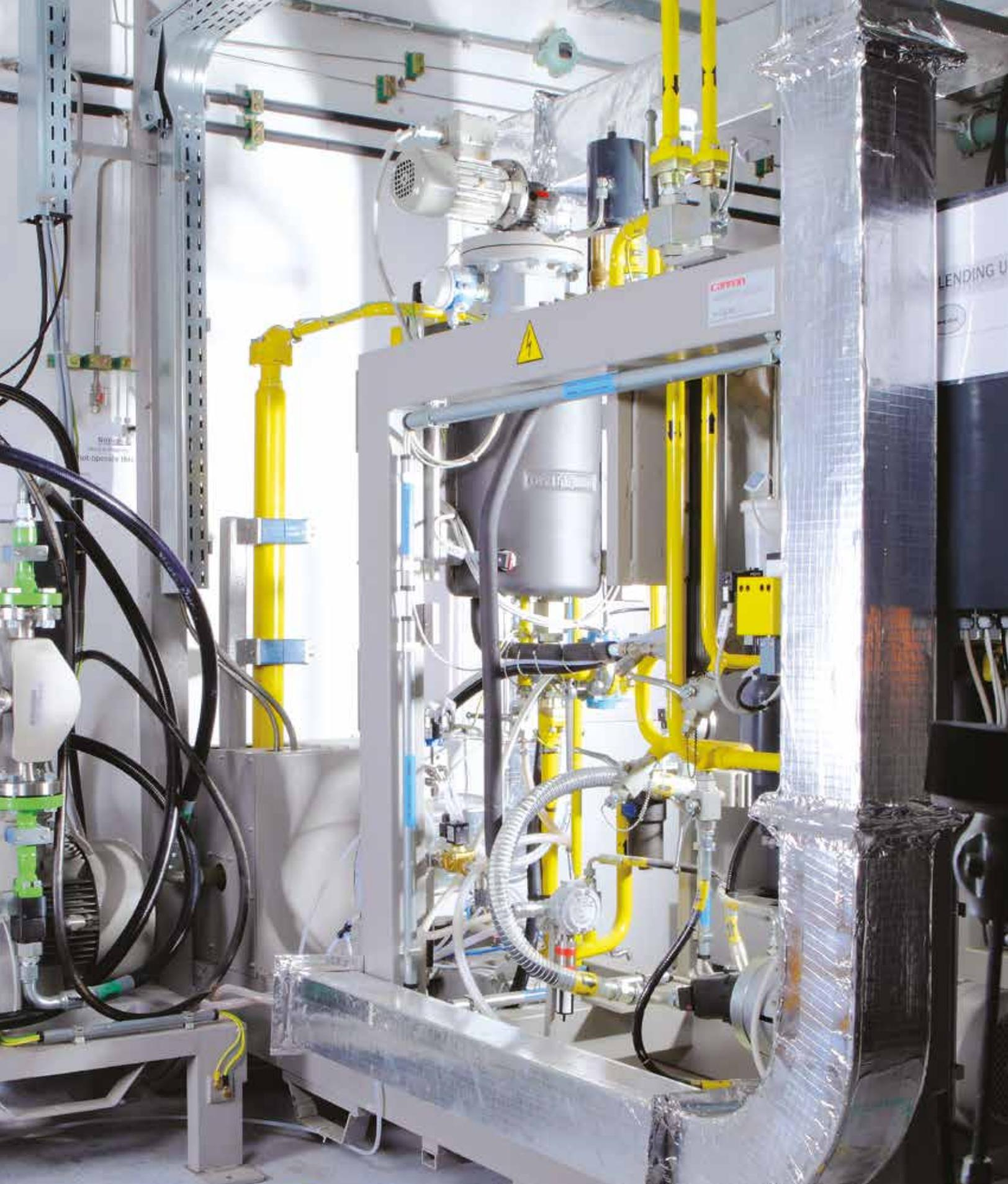
*Our high-pressure foam machines are capable of handling flammable blowing agents and can replicate appliance, panel, and pour-in-place operations. This one is located in our India Technology Center in Gurgaon.*
