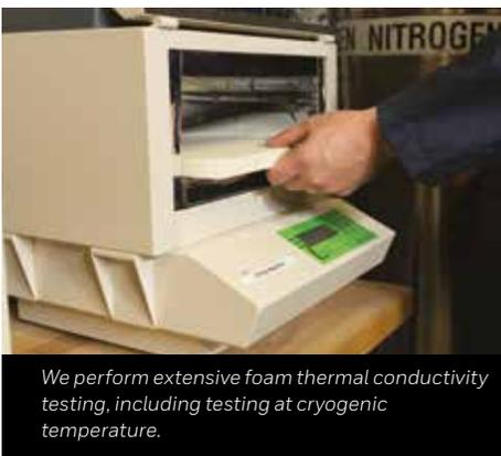
*We perform extensive foam thermal conductivity testing, including testing at cryogenic temperature.*
