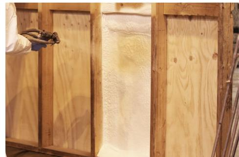
The system was sprayed on a wall assembly to test properties and evaluate the performance of Solstice LBA in the formulation.
