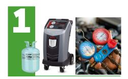
Remove remaining R-134a charge from the vehicle
