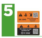
Attach new labels to identify that the refrigerant change has been made
