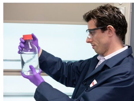
Image shows Solstice LBA being dispensed into an open container. NOTE: Solstice GBA MUST be dispensed into an appropriate pressure-rated container or process line of a closed system.
