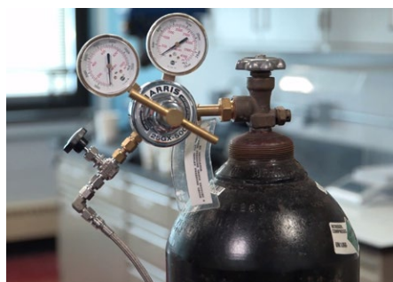
A two-stage nitrogen regulator is required.
