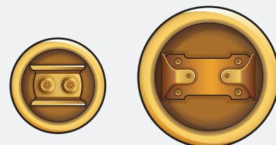
Typical \frac{3}{4} in. solid drum closure
